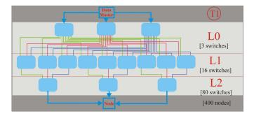
For ≈2000 WR nodes connected to two layers of switches, 15 switches in L0, 80 in L1 and 400 in L2 are required (total 495)
